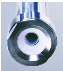
Powder is fluidized as air passes through a small porous disc at the bottom of the outer pick-up tube.
